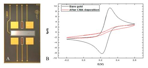
**Figure 1.** (**A**) Biosensor platform containing four gold WE, reference electrode (RE) based on Ag/AgCl and counter electrode (CE) based on platinum (**B**) Cyclic voltammograms of gold WE before (black) and after (red) CMA deposition.
