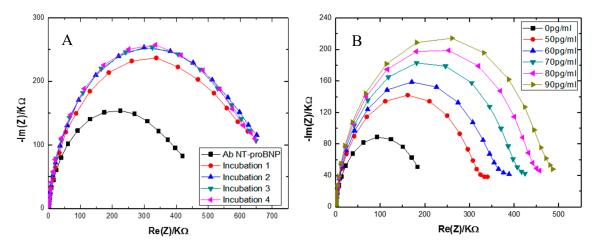
**Figure 2.** (**A**) EIS analyses for biosensor after several incubations in AS. (**B**) EIS analyses for biosensor after several incubations in AS spiked with different NT-proBNP concentrations (50–90 pg/mL).
