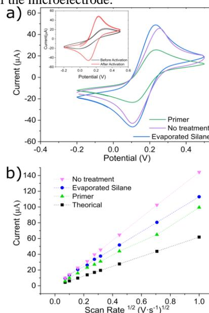
Figure 3: a) Cyclic voltammetry of three microelectrodes printed in the three different treated substrates. Inset shows the behavior of CV before and after activation. b) Correlation of the theoretical versus experimental  $I_p$  in function of square root of the scan rate using the Randles-Sevcik equation.
