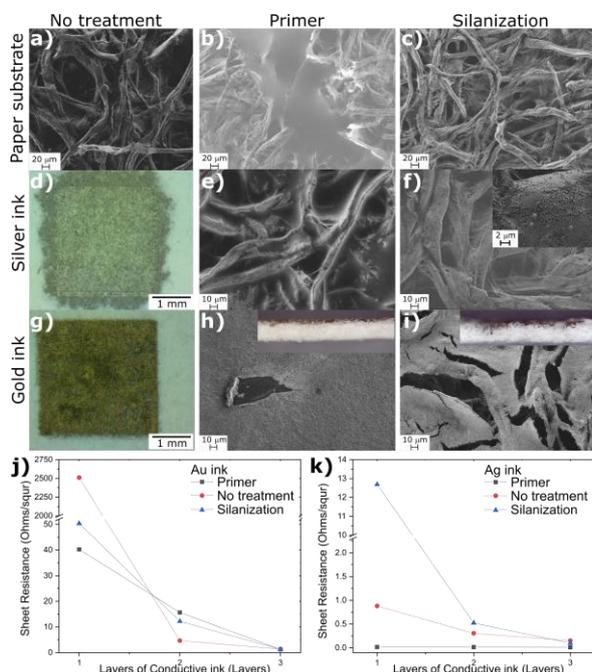
Figure 2: SEM images of paper no treatment a) primer b) silanized c), silver ink on paper no treatment d) primer e) silanized f), gold ink on paper no treatment g) primer h) silanized i). j) and k) sheet resistance vs numbers of layers deposited.
