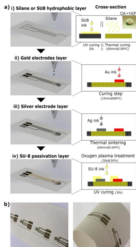
Figure 1: a) Fabrication steps of the three-electrode array based on inkjet printing with printing of the primer layer or evaporation of silane, printing of the gold and silver elements and printing of the passivation layer after thermal sintering and plasma treatment, b) photographs of the final device.
